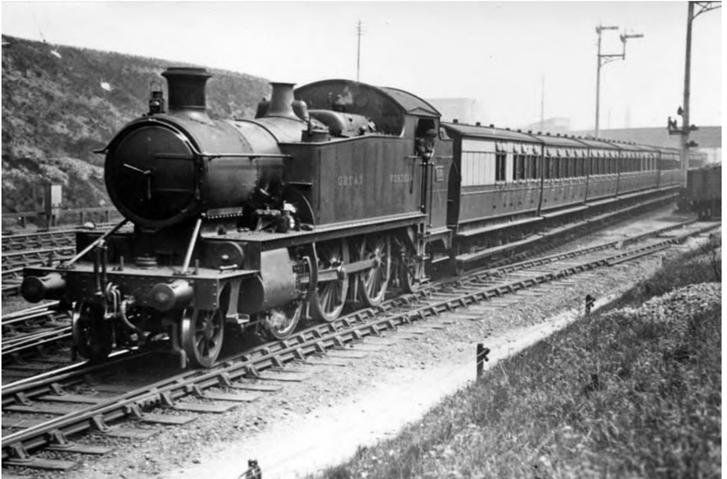
GWR 3100 Class 2-6-2T No 3138 on a Birmingham Snow Hill to Stourbridge Junction service.
