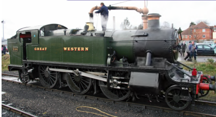
The difference in size between Large and Small Prairie Tanks is evident in these photos of 5164 and 4566 taking water on the Severn Valley Railway
