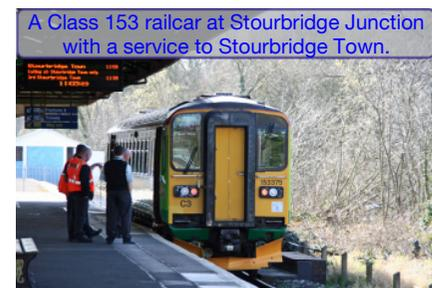
This class was a modification of a Class 155 two car unit with each coach given an extra cab and driving gear. Class 153 units still exist on the UK rail network and either work on short rural lines in isolation or are coupled with other Sprinter sets to strengthen them when required. A Class 153/170 combination is often employed on the Stourbridge Line, while Class 150/153 combinations are regularly seen on the Great Western Railway network.
